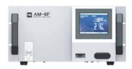
Fully Automated, Continuous Mercury Monitor, the AM-6F is designed to measure gaseous elemental mercury (GEM) from ambient air accurately down to the sub nano-gram per cubic-meter level. The technique used is Direct Gold Amalgamation Sampling - CVAFS (Fluorescence technology) Detection.
